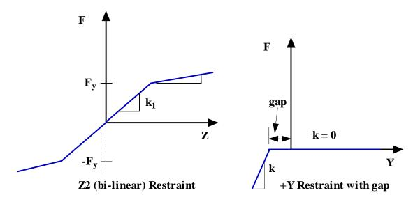
Note that rotational restraints may also be linear or nonlinear in a similar manner. The stiffness in these cases relate a moment to rotation resulting in a stiffness in units of Ft-lbs/degree (length\*force/angle).
